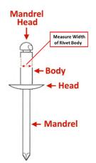
To determine the correct nose piece, measure the width of the rivet body. Once rivet size is determined use the corresponding nose piece (2.4mm, 3.2mm or 4mm) which is stamped on the side of the nose piece.
